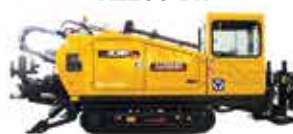
Motor: Cummins QSB6.7-C220 TIER III Bomba hidráulica: Sawyer Danfos
