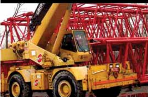
Grove RT635C, S/N 84957, 1997, 35 Ton, Cummins Diesel, lança principal 105' (32,0 m), braço 51' (15,5 m), Unidade 6275. US$135.000,00
