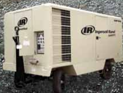
XHP 900 WCAT 900 cfm (25.5 m 3 /min) 350 psig (24.1 bar)
