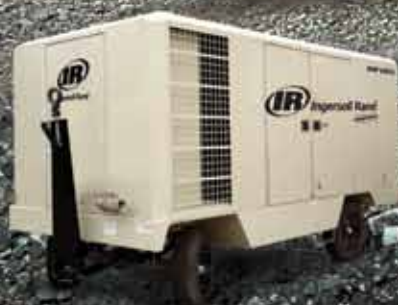
XHP 1070 WCAT 1.070 cfm (30.3 m 3 /min) 350 psig (24.1 bar)
